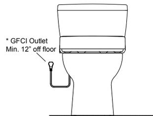
\* The 3-prong cord on the Washlet is on the left side and is 3' long. The GFCI outlet needs to have 120V, 10amps.
