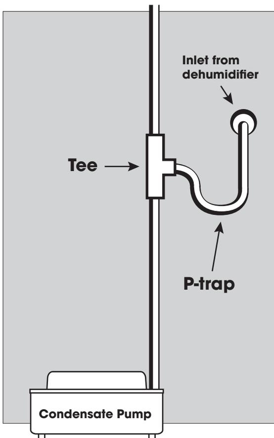
Thank you for your purchase of this condensate pump. This pump is not only designed for use in air conditioner applications but also with dehumidifier. To ensure this pump operates properly, please be aware of this information. This condensate pump is designed for condensate water up to 140°F continuously. When using this pump with a de-humidifier, please install a P-trap in the condensate drain line before the pump to help ensure correct operation.
