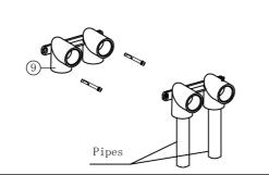
3. Connect  ${\rm G1/2}$  connector to Inwall Body with PTFE tape, ensure connector outside the wall no leakage and keep in horizontal level.
