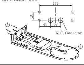
$6.\, Tighten$  screws No. 5, connect two hoses to G1/2 connector No. 6 and guaratee no leakage. Cut the end of PTFE taped connector by cutting machine if need to make connector shorter and repeat installation from step 3.
