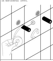
$4.\,\mathrm{Unscrew}$  the seven M4 screws with Allen Key, Slip out the wall cover No.2 and then put out the Backcover No.3.
