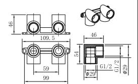
2. Connect pipe to inwall body, Drill holes and use two wall mounting screws to fit the Inwall Body. Seal wall if no leaking after water test.
