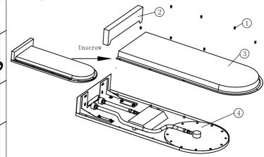
5. Drill the following holes according to location of G1/2 connector, and then fasten shower head mainbody No. 4 by Expansion screws.
