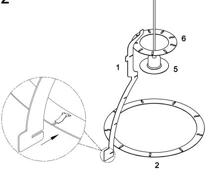
Attach part (1) to ring (5,6, 2) as per diagram.
