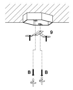
Use screw (B) to secure the metal bracket (9) to the ceiling mount as per diagram.
