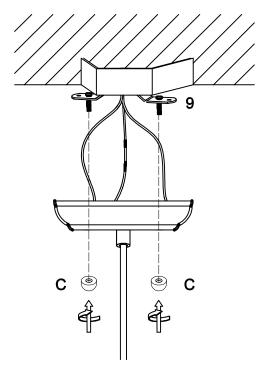
Use nut (C) to secure the light to the metal bracket (9) as per diagram. Coil wires safely to ensure proper fit.
