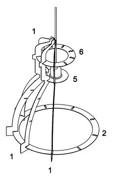
Attach 3 additional part (1) to ring (5,6, 2) as per diagram.
