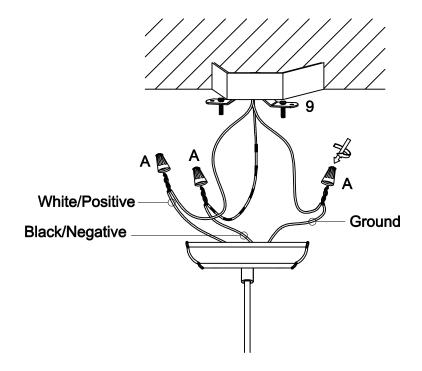
Use the wire nut (A) to secure the wires as per diagram.
