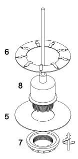
Assemble parts (7, 5, 8, 6) as per diagram.
