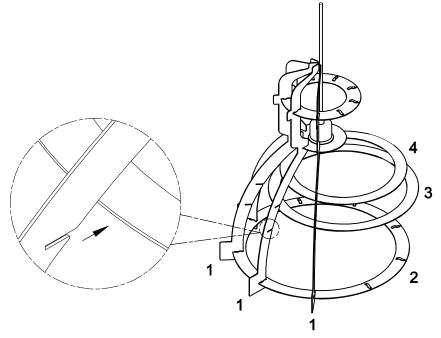
Attach rings (3, 4) to part 1 as per diagram.
