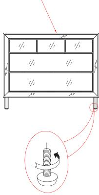
Adjust leveler if needed to level the chest on uneven floor.
