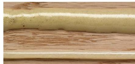
Unlike alternative adhesives (top), 3M™ 5010 Polyurethane Multi-Purpose Adhesive (bottom) exhibits almost no foaming or line expansion.
