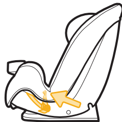
Lower Anchor Belt Storage Location
