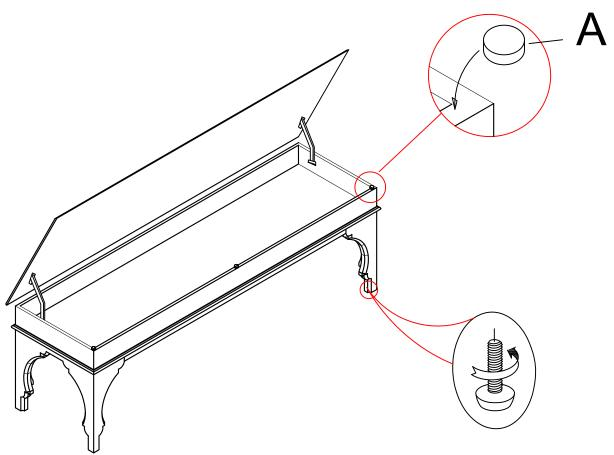
Adjust leveler if needed to level table on uneven floor.
