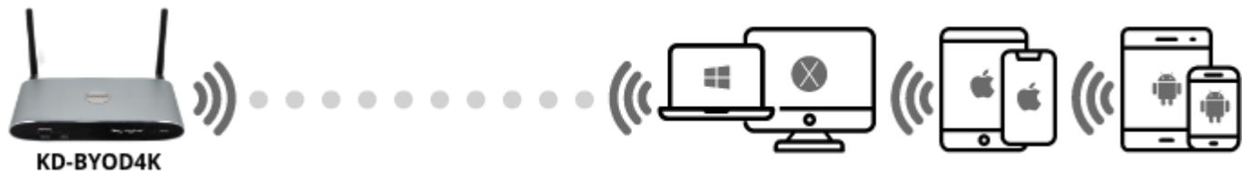
**LAN Connect Mode** requires KD-BYOD4K be wired into your local network. Wireless devices access KD-BYOD4K via your existing external WiFi network therefore allowing users to stay connected to an internet enabled network(s). WiFi Direct mode is disabled when LAN Connect Mode is enabled.
