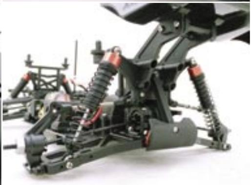
Suspension is similar to Helion's Short Course version, fully independent long stroke oil filled coil over
