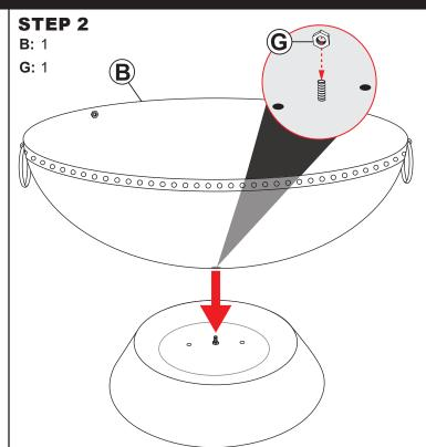
Align the center hole in Fire Bowl (B) with the bolt on Fire Bowl Base (C). Secure the bowl and base by hand-tightening M10x35mm Nut (G).
