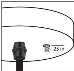
NOTE: Position cross bar to junction box to determine the adjustment length of screw based on junction box being level (recessed or sticking out from ceiling). Momentarily place canopy over cross bar and make sure screws are protruding 0.25 inches from canopy.
