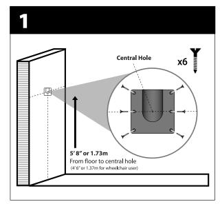
On the wall, mark a spot 5'8" from the floor and align the central hole of **Part A** with the mark. Drive the **6 Mounting Screws** into the corresponding holes. Use the **6 Wall Anchors** if not over a stud.
