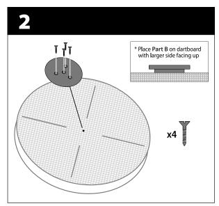
Apply **Part B** directly in the center on the backside of your dartboard. Drive the **4 Stabilizer Screws** into the proper holes.
