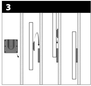
After **Part A** and **Part B** have been installed, slide the dartboard onto the **QuickFit Dartboard Mounting Bracket**.
