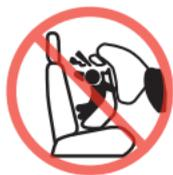
**NEVER** install a rear-facing child restraint in the front seat of a vehicle equipped with an active frontal airbag.
