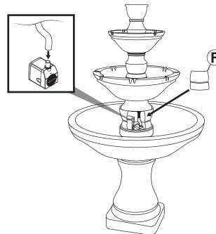
Firmly connect the water tube to the pump.
