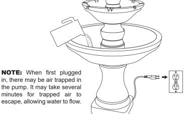
Fill each tier with enough water to keep the pump fully submerged during operation, approximately 7 gallons (26.5L) total.
