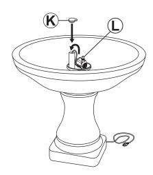
Place Pump (L) in the center of the bottom bowl and run the power cord down the built-in tube and out under the groove in the bottom of the pedestal. Install Leak Guard (K) over the tube.
