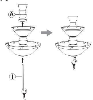
Run the longer side of Water Tube (I) up through the PVC tube and connect it to Topper (A).
