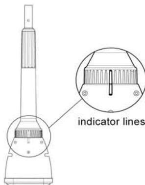
It is very important to make sure the unit is sealed and in the on position before submerging. **Do not submerge the unit until indicator lines meet.** Your cleaner should never be left in the water when off, as leakage can occur.
