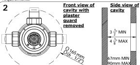
At this stage ENSURE the ROUGH is correctly installed (In-Wall) - Valve Body: U.5585R (pictured above & left), before attempting this Trim installation.
