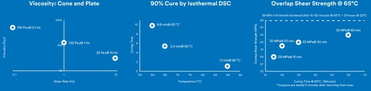
\*Data generated with 3M internal testing using 3M<sup>™</sup> Scotch-Weld<sup>™</sup> One-Part Epoxy Adhesive 6102 (Black). For more specific details consult the <u>Technical Data Sheet</u>.
