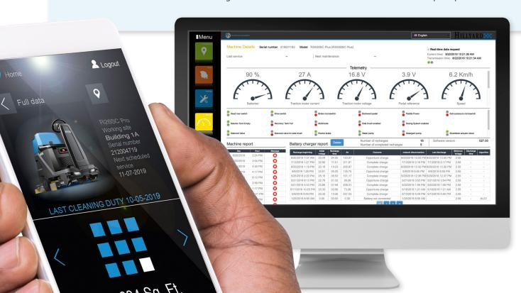
An authorized Hillyard Trident Service Center can view real-time telemetry data, diagnose systems, and update settings over the internet - keeping your equipment running at peak performance - and minimizing downtime.
