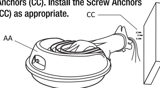
**3** Feed the power supply wires into the conduit fitting and connect with Area Light Fixture (AA) wires; Ground to Ground, Neutral to White and Hot to Black. Mount the Area Light Fixture (AA) housing to the wall as appropriate.
