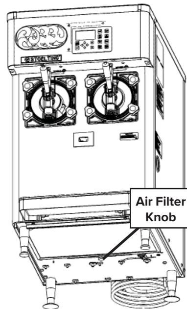
Figure 3-7 E122 Condenser Filter Removal
