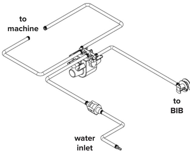
Figure 2-2 Auto Fill Pump Tubing Layout
