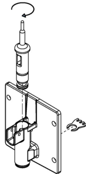
**Figure 3-5 Spigot and Ice Breaker Bar Removal**
