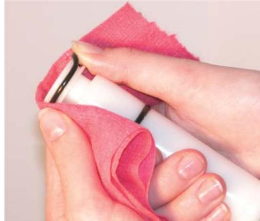
**Figure 3-4 Removing O-Ring**
