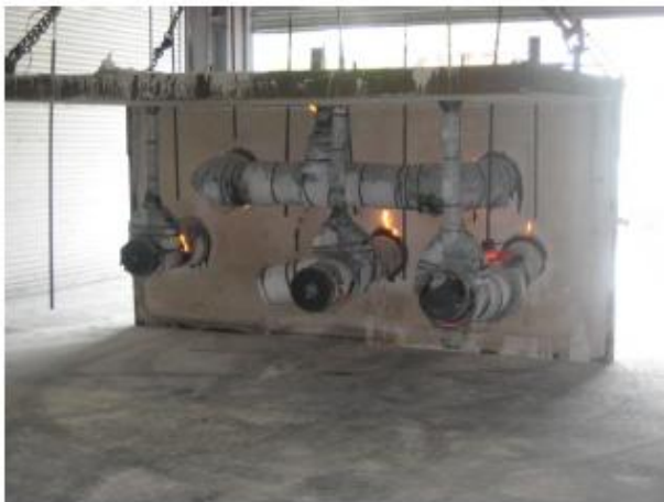
Figure 4-3 Test Assembly Prior to Initiation of Hose Stream Test
