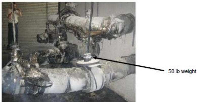
Figure 4-12 Specimen C Following Hose Stream Test
