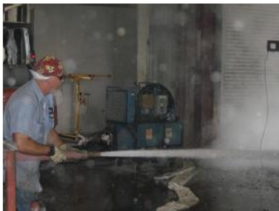
Figure 4-3 Test Assembly Prior to Initiation of Hose Stream Test
