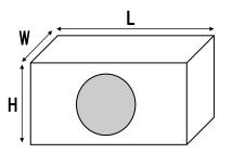
**Sealed Dimensions:** Length (L) : 16" (406 mm) Width (W) : 9" (229 mm) Height (H) : 12" (305 mm) Cutout Diameter: 9-1/8" (232 mm) Int. Volume: 0.6 ft<sup>3</sup>
