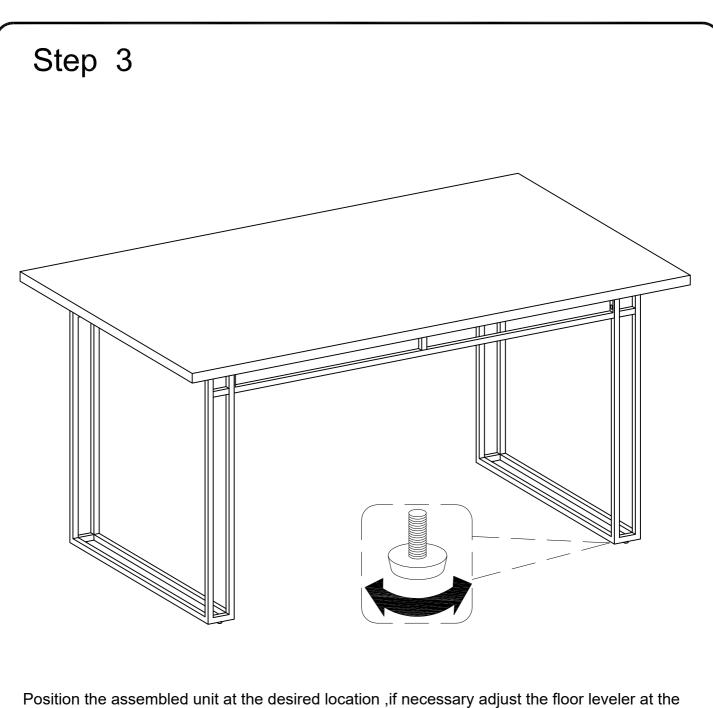
Position the assembled unit at the desired location ,if necessary adjust the floor leveler at the bottom of the leg to level the unit .
