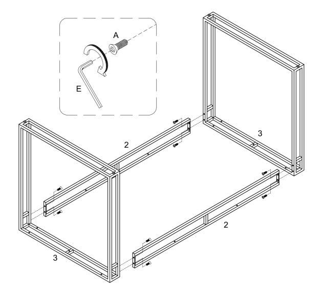
Using bolt (A) attach parts (3) to part (2) with Hex key (E) as per diagram.
