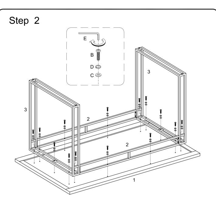
Using bolt (B) attach Lock washer (D) and Flat washer (C) into parts (2,3) to part (1) with Hex key (E) as per diagram.
