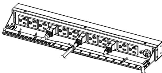
Use the Cable Ties provided to fasten each power cord to the Cord Retention Tray.
