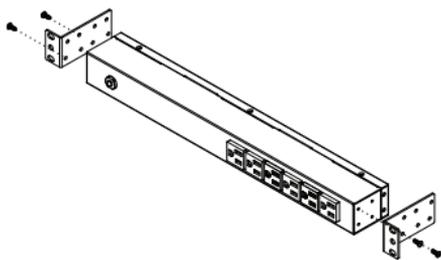
Install the screws (M4 X 6) in holes diagonal from each other.
