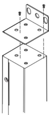
Install the screws (M4 X 6) in holes diagonal from each other.
