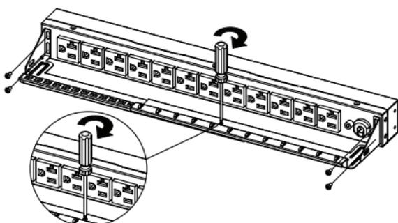
Attach the Cord Retention Tray to the PDU with the 4 supplied Cord Retention Tray Mounting Screws (M3 X 6). Tighten the Cord Retention Tray with the screw on it.
