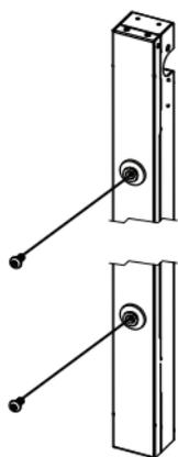
Attach the Keyhole Mounting Pegs to the PDU with the 2 supplied Bracket Mounting Screws (M4 X 6).
