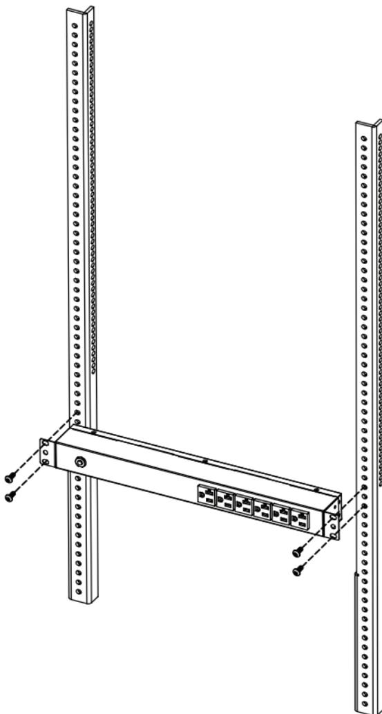
Install the PDU using fasteners compatible with the rack.
