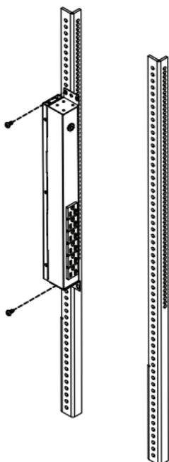
Install the PDU using fasteners compatible with the rack.
