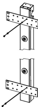
Attach the Vertical Mounting Brackets to the PDU with the 4 supplied Bracket Mounting Screws (M4 X 6).
