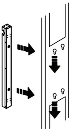
Align the the Keyhole Mounts to the Keyhole Slots on the rack. Insert and slide down to lock firmly into place.
