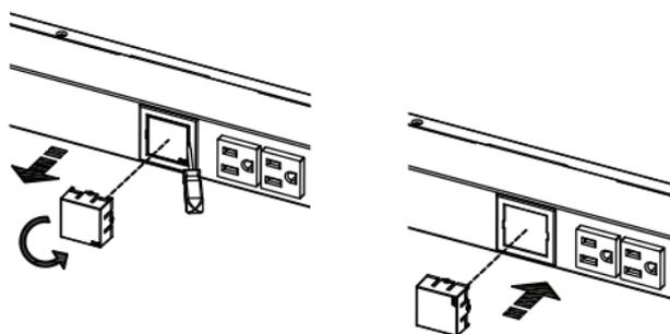
Use a screwdriver to gently remove the LED Meter. Rotate the LED Meter 90 degrees, and insert back into the PDU.
