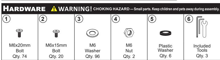
**! HELPFUL HINT:** Do not tighten hardware until all components have been loosely assembled. If the hardware is tightened too soon, mounting holes may not align, and parts may not easily fit together.
