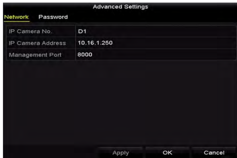
Figure 2-33 Network Configuration of the Camera
