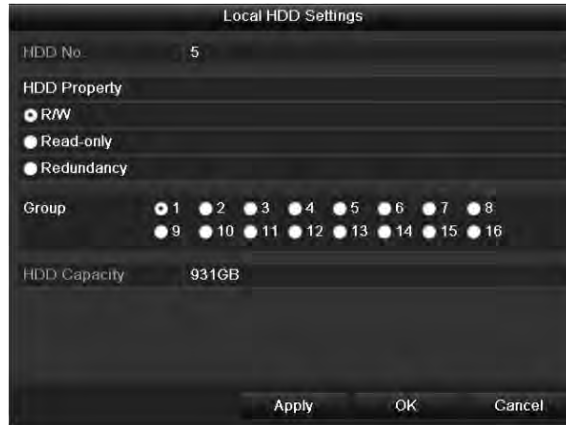
Figure 12-13 Local HDD Settings Interface
