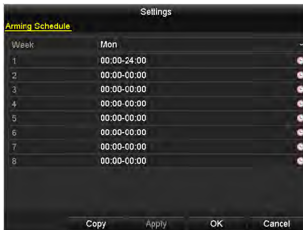
Figure 8-17 Set Arming Schedule of Alarm Output
