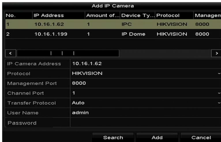
Figure 2-26 Quick Adding IP Camera Interface
