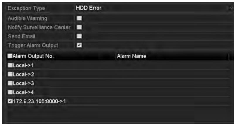
Figure 12-27 Configure HDD Error Alarm
