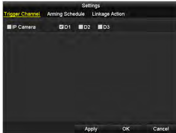
Figure 8-2 Set Trigger Camera of Motion Detection
