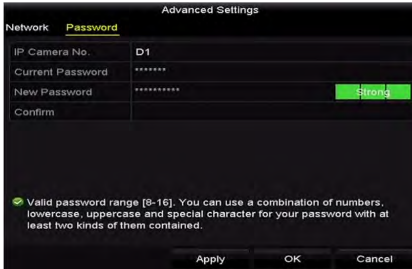
Figure 2-34 Password Configuration of the Camera
