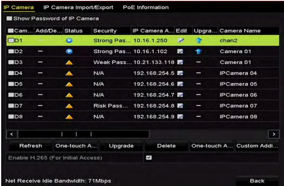
Figure 2-27 Adding IP Camera Interface
