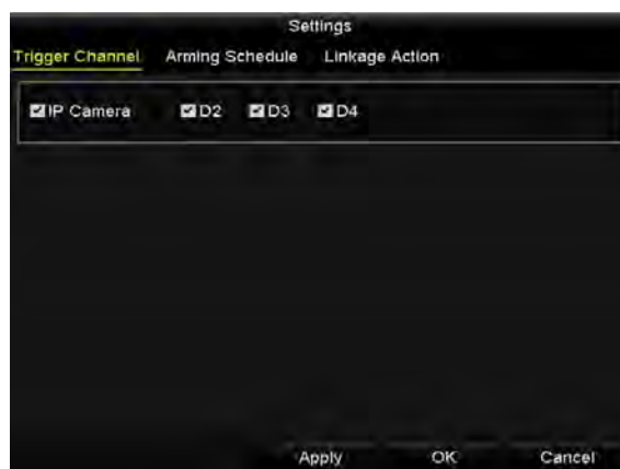
Figure 5-18 Set Trigger Camera of VCA Alarm
