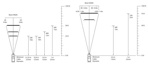
CDM-50 Measurement versus Cable Diameter
