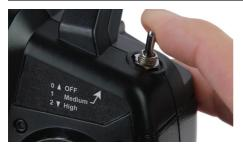
The Mini Gamma is equipped with a three-position, 6-axis gyro-assisted flight stabilzation control that reduces the control sensitivity for beginners, limits the airplane's angle of bank and helps dampen the effects of wind and turbulence during a flight. The three positions are:
