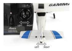
Check that the elevator operates in the correct direction. Pulling the elevator stick back should cause the elevator to move up in response. Pushing the elevator stick forward should cause the elevator to move down in response.
