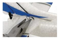
Check that the rudder operates in the correct direction. Moving the aileron stick to the left should cause the rudder to move left in response. Right aileron stick will move the rudder to the right.
