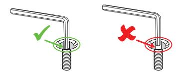
**TIP:** Always fully insert the hex key inside the designated notch of the bolt.
