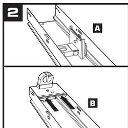
**A** Place track assemblies into slots in the end of channel.
