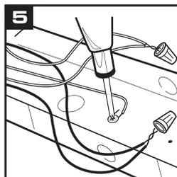
With power off, make power supply connections as shown. Attach ground wire to green ground screw, connect power supply.
