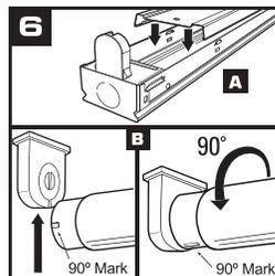
**A** Align channel cover and push down to snap into place.
