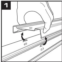
Squeeze channel at markers shown to remove channel cover.
