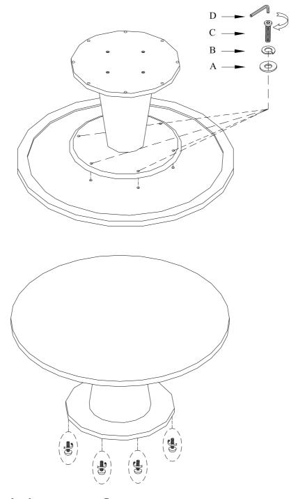
Adjust levelers if needed, to level case on uneven floor
