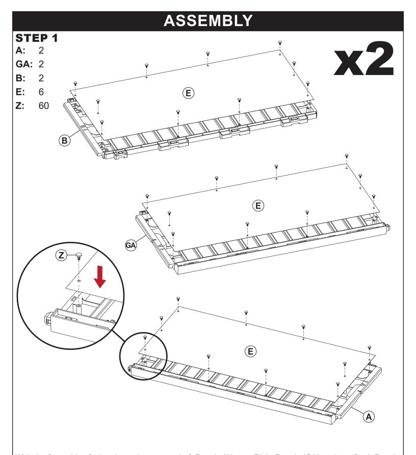
With the front sides facing down, lay out two Left Panels (A), two Right Panels (GA) and two Back Panels (B).
