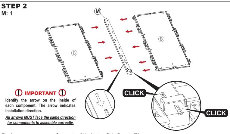
Firmly connect one Long Connector (M) with two Side Panels (B).
