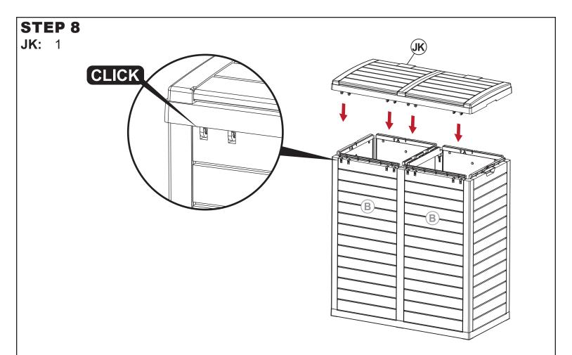
Firmly but carefully press the tabs on Lid (JK) into the grooves on the back panels until they snap in place.
