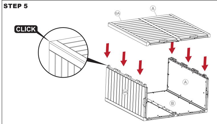
Ensuring the arrows on the insides of all panels are facing the same direction, firmly and evenly press the front panels onto the side panels, as shown.
