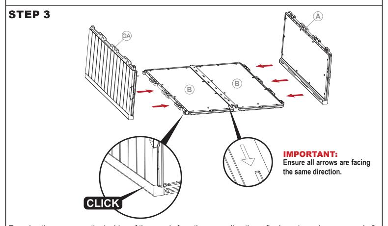
Ensuring the arrows on the insides of the panels face the same directions, firmly and evenly press one Left Panel (A) and one Right Panel (GA) onto the back panels.
