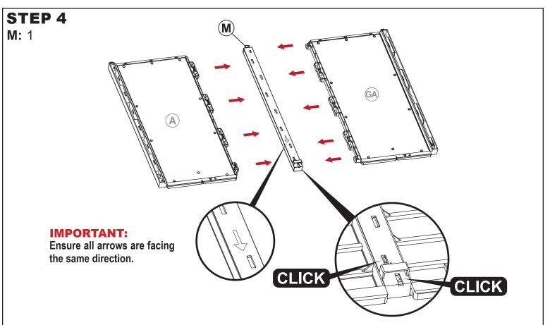
Firmly connect one Long Connector (M) between Left Panel (A) and Right Panel (GA).
