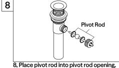
8. Place pivot rod into pivot rod opening. Slide pivot nut over pivot rod and thread it on the drain body. Tighten firmly.
