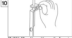
10. With lift rod in position on the faucet, insert lift rod through lift rod strap and secure with the clevis screw.
