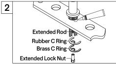
2. Sparingly apply a small bead of silicon caulking around the center hole on top of the sink (do not use Plumber's Putty as it may damage finish and void warranty). From the top of the sink insert the spout through the center hole. From the bottom, slip the rubber & brass C rings onto the threaded rod, tighten extended lock nut.
