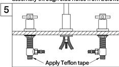
5. After applying Teflon tape attach flex line to outlet port of stem assembly, use caution to not over tighten. Apply Teflon tape to valve stem inlet and Shut-off valves and attach supply lines (not included) to inlet port of stem assembly.
