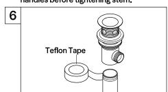
6. Thread mounting nut and bottom gasket onto drain body. Wrap the threaded end of the drain body with Teflon tape.
