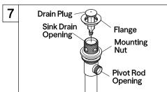
7. Apply silicone to the underside of the flange. Install the flange body up through the drain opening, positioning it with the pivot rod opening facing the back of the sink. While holding it in place, hand-tighten the mounting nut. Be sure to clean off any excess silicone.
