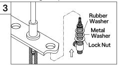
3. Hot and Cold Stem assemblies are easily Identifiable by a Red (Hot) or Blue (Cold) band, thread lock nut and insert metal and rubber washers on stem assembly and insert stem assembly through side holes from below.
