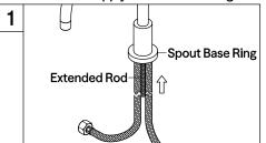
1. Insert spout base ring onto the spout, making sure to line up the notch on the base ring with the groove at the back of the spout, after applying thread dope on the male threads of the supply lines, thread supply lines to the inlets at the bottom of the faucet, thread extended rod to the bottom of the faucet using a Philips head screwdriver.
