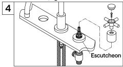
4. While holding from under the sink thread escutcheon on to Stem assembly, install handle and adjust to a suitable height to allow sufficient space for handle to operate smoothly. Tighten bottom nut make sure to align direction of lever handles before tightening stem.
