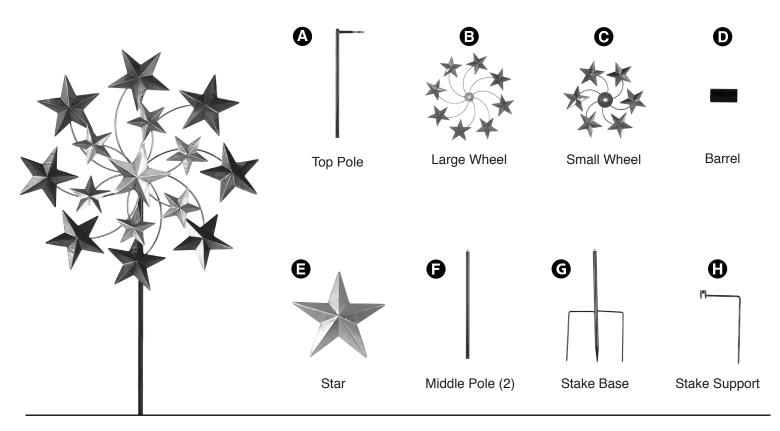
**Step 1:** Attach large wheel (B) to top pole (A) by inserting it through the opening.
