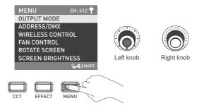
Rotate the "right knob" to select the options, press the "right knob" to enter the corresponding secondary menu,
