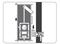
Align the quick release plate on the control unit with the quick release mount on the clamp to mount the control unit on to the clamp.
