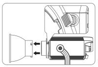
When removing the reflector, push and hold the lock catch and rotate until the reflector is free to be removed from the fixture.
