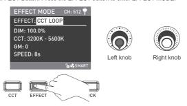
Forza 500B II has built-in effects including CCT LOOP, INT LOOP, FLASH, PULSE, STORM AUTO, STORM MANUAL, TV, PAPARAZZI, CANDLE/FIRE, BAD BULB, FIREWORK, EXPLOSION AUTO, EXPLOSION MANUAL and WELDING.
