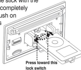
**Step 2** Pull out the iPod docking as shown below.
