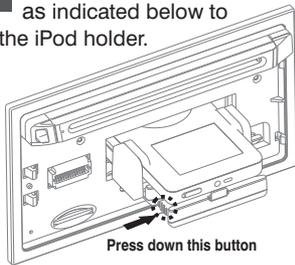
**Step 7** Push on the iPod holders on both sides until they stop.
