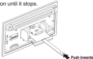
**Step 3** Press on this button on the left side as indicated below to unlock the iPod holder.
