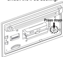
**Step 5** Once the stick with the connected iPod is completely out, user should push on the locking buttons on the both sides of the iPod connector to release the iPod as indicated in the picture, and remove the iPod unit.
