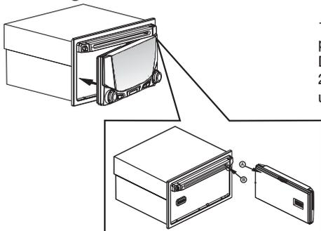
1. Attach the panel at the right side first, with point B on the main unit touching point A on the D.C.P. (As shown on the diagram).
