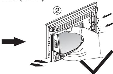
Slightly lift up the panel & pull out the panel side way in order to remove the front panel.
