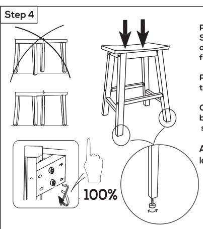
Put chair in the upright position and SIT ON THE CHAIR to press downwards on the seat pad ensuring that all 4 feet touch the ground and chair is leveled.
