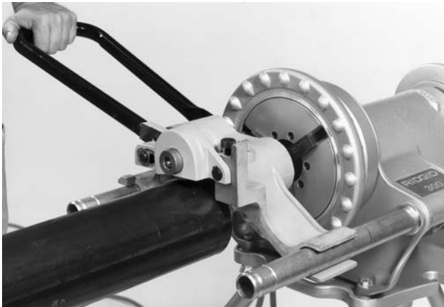
Figure 12 – Forming the Roll Groove
