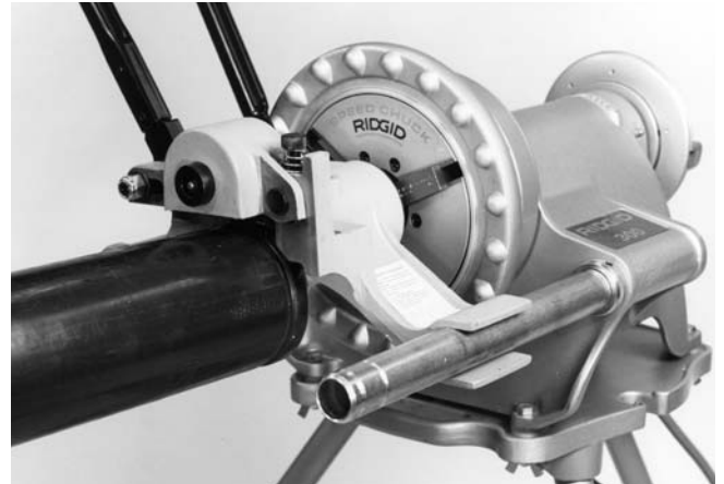
Figure 9 – Feed Handle in UP Position
