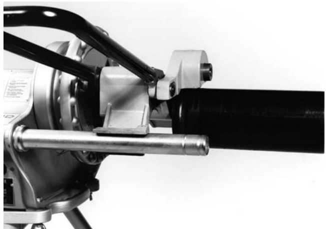
Figure 6 - Square Pipe & Pipe Support
