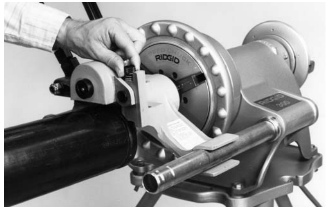
Figure 10 – Loosen Depth Adjustment Screw
