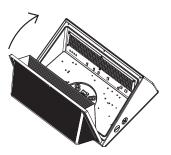
Close the Front Cover and secure with the Front Cover Screws (BB).
