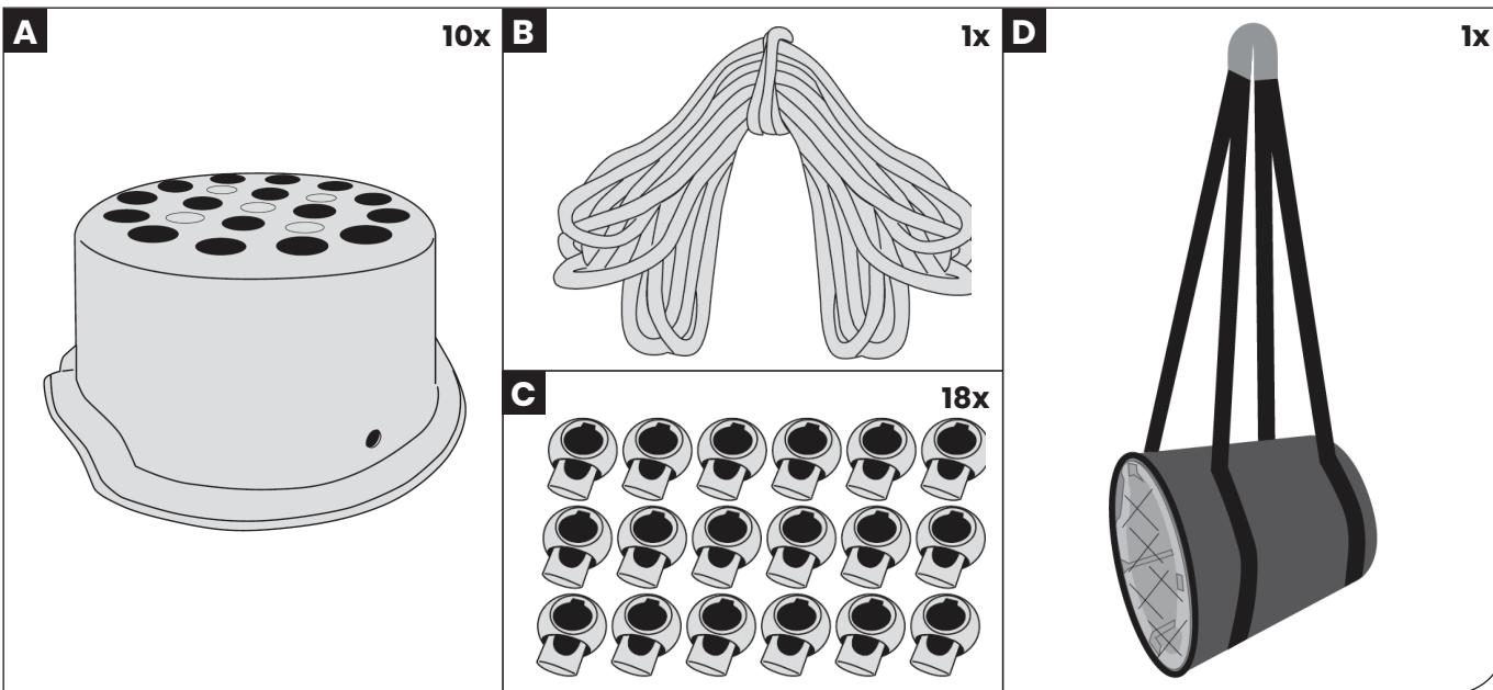
Optional rope is marked at 1" intervals for spacing. Adjustable locks keep buckets in place.
