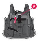
Make sure the anchor is completely through the front slot and is lying flat against the bottom of the seat.
