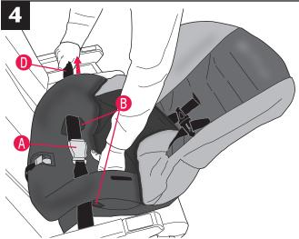
The aircraft seat belt (a) must be as tight as possible. Route the excess seat belt strap (D) back through the rear-facing belt path (B) opening, as shown above. Using your full weight, push the child restraint firmly onto the aircraft seat while pulling on the excess seat belt strap to tighten.
