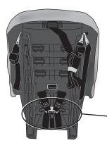
Attach the harness straps <sup>(3)</sup> to the splitter plate <sup>(9)</sup> using the *infant position* (page 37) on the harness straps. As your child grows, you can attach the harness straps <sup>(3)</sup> to the splitter plate using the pockets at the end of the
