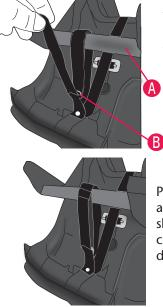
When the recline stand is in the **recline position**, wrap Velcro<sup>®</sup> strap around the recline stand (A) and insert the end of the strap through the D-ring (B), as shown.
