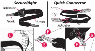
Refer to your vehicle owner's manual to locate the lower anchor bars (a) on your vehicle seat. Attach the right hook (b), or clip (c), to the right anchor bar (c) and the left hook, or clip, to the left anchor bar. **DOUBLE CHECK** that the lower anchor connector hook is fully engaged by pulling hard on the lower anchor connector strap.
