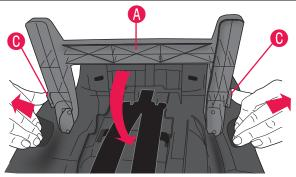
To fold the recline stand (a), turn the child restraint upside down. Pull the shell walls away from the locking tabs (b) on the sides of the recline stand and rotate the recline stand downward until it lies flat, as shown.
