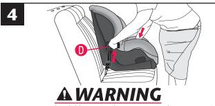
**DO NOT** use this child restraint if it moves more than 25 mm (1 in.) side-to-side or front to back at the forward-facing belt path. Serious injury or death may result from poor installation. If you can not tightly secure the child restraint, try again, move it to another location, or install with the vehicle seat belt.
