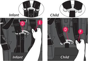
There are two positions on the harness straps. The top loop (2) is for infant use. The bottom loop (2) is for use as your child grows. Reattach the harness strap onto the splitter plate (1). Repeat on the other side.
