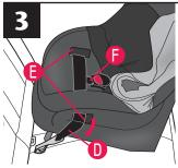
Pull the seat pad off of the front of the child restraint. Route the Lower Anchor Connector strap and hook through the rear-facing belt paths (2). *IMPORTANT: Make sure the Lower Anchor Connector strap is in front of the crotch strap and it lies flat without twisting, as shown. Reconnect the seat pad to the front of the child restraint.*
