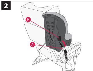
Route the aircraft seat belt () through the forward-facing belt path opening in the back of the child restraint and continue through the belt path opening () on the opposite side of the child restraint.
