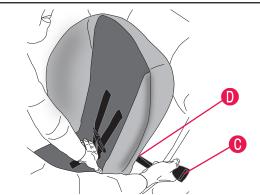
The aircraft seat belt must be as tight as possible. Route the excess aircraft seat belt strap <sup>()</sup> back through the forward-facing belt path <sup>()</sup> opening, as shown above. Using your full weight, push the child restraint firmly onto the aircraft seat while pulling on the excess seat belt strap to tighten.
