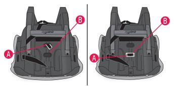
To reposition the crotch strap, first turn the child restraint upside down. Turn the crotch strap harness anchor (A) sideways and push it through the slot in the bottom of the seat shell (B).
