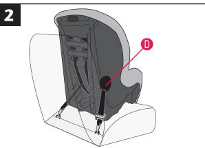
Adjust the child restraint to the **upright position** (page 38) and place it in your vehicle **forward-facing**, as shown. Route the Lower Anchor Connector Assembly through each side of the forward-facing belt path **1**. **Note:** Lift seat pad away from seat for easier access. Make sure Lower Anchor Connector Assembly strap lies flat without twisting.
