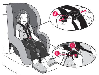
Push the release button () and pull the chest clip apart. Press the red buckle release () and remove the buckle tongues ().
