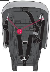
When the Lower Anchor Connector assembly is not in use you **MUST** attach the hooks <sup>(b)</sup> to the back of the child restraint. A loose Lower Anchor Connector assembly strap and hook may injure your child.
