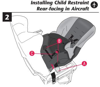
Pull the seat pad off the front of the child restraint. Route the aircraft seat belt (a) through the rear-facing belt path (b) opening on one side and continue through the belt path opening on the opposite side of the child restraint, as shown above.
