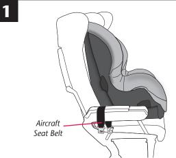
Adjust the child restraint to its **upright position** (page 38), then place it on the aircraft seat **forward-facing**, as shown above.
