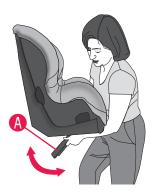
Lift the child restraint and flip the recline stand (3), located under the child restraint seat, to either the **upright** or **recline position**.
