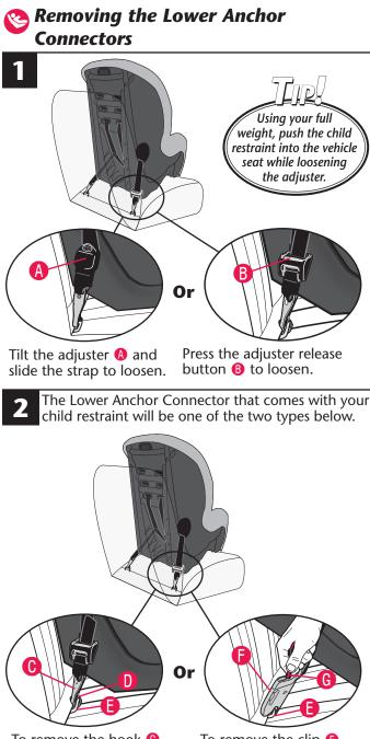
To remove the hook (9, press the tab (1) and twist, then remove from anchor (2).
