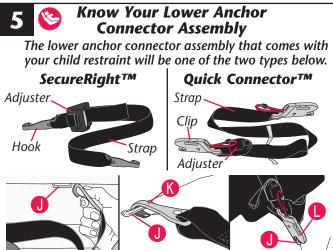
Refer to your vehicle owner's manual to locate the lower anchor bars **1** on your vehicle seat. Attach the right hook **3**, or clip **1**, to the right anchor bar **1** and the left hook, or clip, to the left anchor bar. **DOUBLE CHECK** that the lower anchor connector hook is fully engaged by pulling hard on the lower anchor connector strap.
