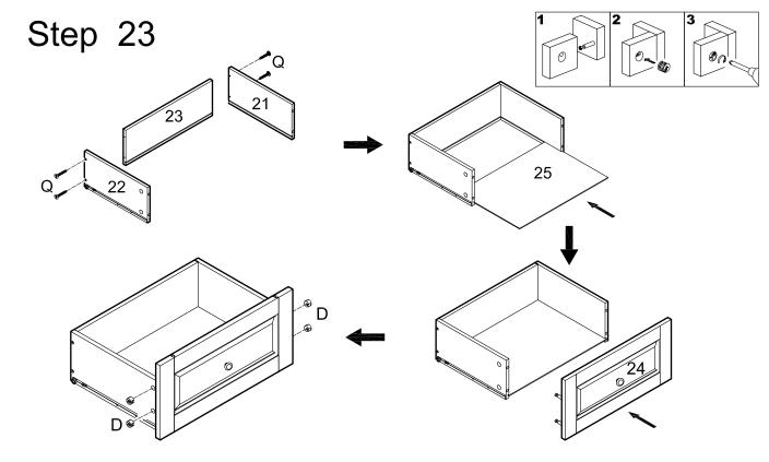
Attach drawer sides (21,22) to drawer back (23) using extra-large screws (Q). Slide drawer bottom(25) into the drawer assembly. Attach drawer front (24) to the drawer assembly using cam bolts as guides. Insert small cam locks (D) into drawer sides (21,22) and tighten with a screwdriver.
