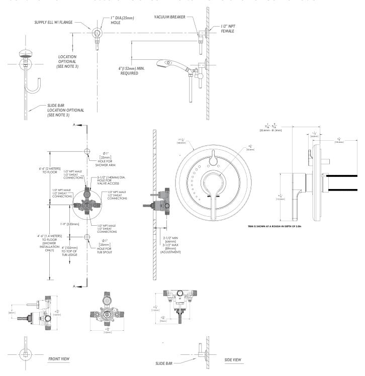
NOTE: 1. All dimensions are in inches (millimeters) unless otherwise specified and are subject to change without notice. 2. Unless otherwise specified, all inlets and outlets are 1/2" female copper sweat. 3. For ADA mounting locations, consult ADAAG, ANSI A117.1, or static regulations
