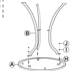
Install three Grub Screws (H) into Tabletop (A). Loosely install three Table Legs (B) using Washers (I) and Nuts (J).
