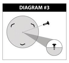
Drive the Dartboard Mounting Screw into the pre-drilled center hole, leaving space to hang the dartboard onto the Mounting Bracket.
