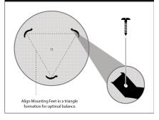
Apply the Mounting Feet to the backside of your dartboard, spaced evenly around the perimeter, driving the Stabilizer Screws into the proper spots.
