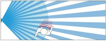
PIR sensors monitor the patterns of background heat energy in a given space. That is, if you sit still for a long time, the sensor will think of your static heat signature as a normal condition and return to "Off" mode. When a movement of a heat source is detected the sensor turns "On". When the sensor does not detect the heat source movement it returns to "Off" mode. PIR sensing technology is great for avoiding false triggers.
