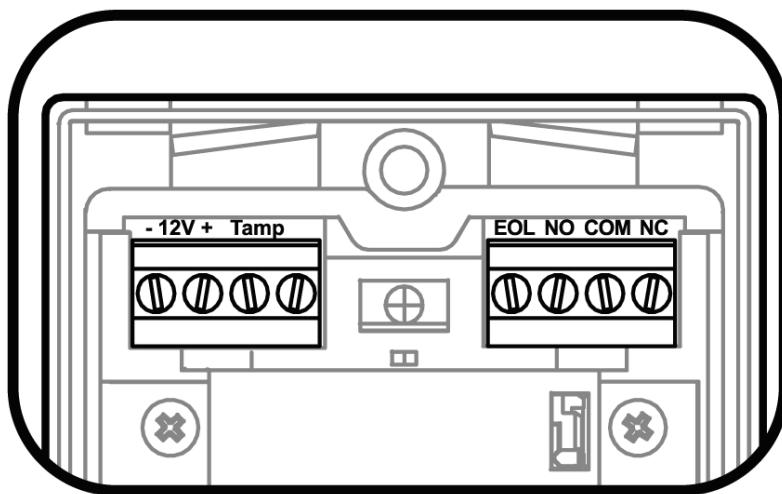
**Terminal 1 - Marked “-” (GND)** - Connect to the ground of the Control Panel.
