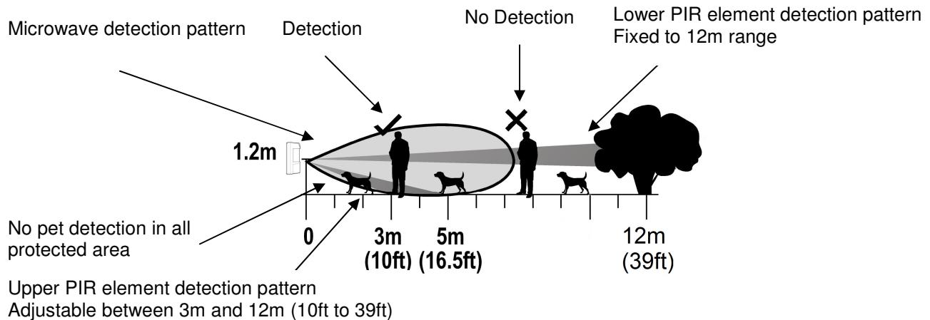
The LC-171 can differentiate between pets and human bodies and alert accordingly by having microwave movement detection combined with two PIR detection beams:.
