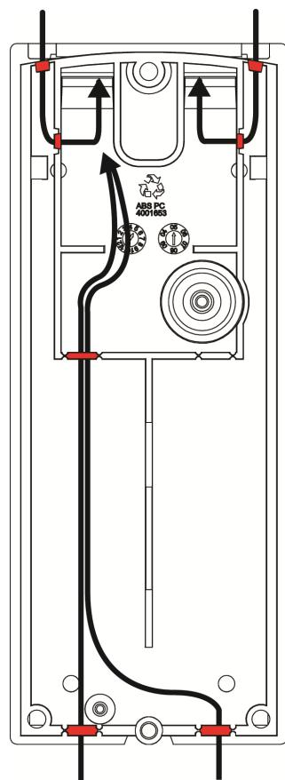
10. Attach the sealing "U" shaped Sponge Pad to the wire opening from the rear side after the wires have been connected and prior to final product affixing to the mounted bracket.
