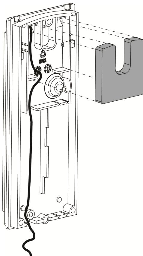
11. Place the detector on the mounting bracket from top side down and then lock the screw at the bottom.
