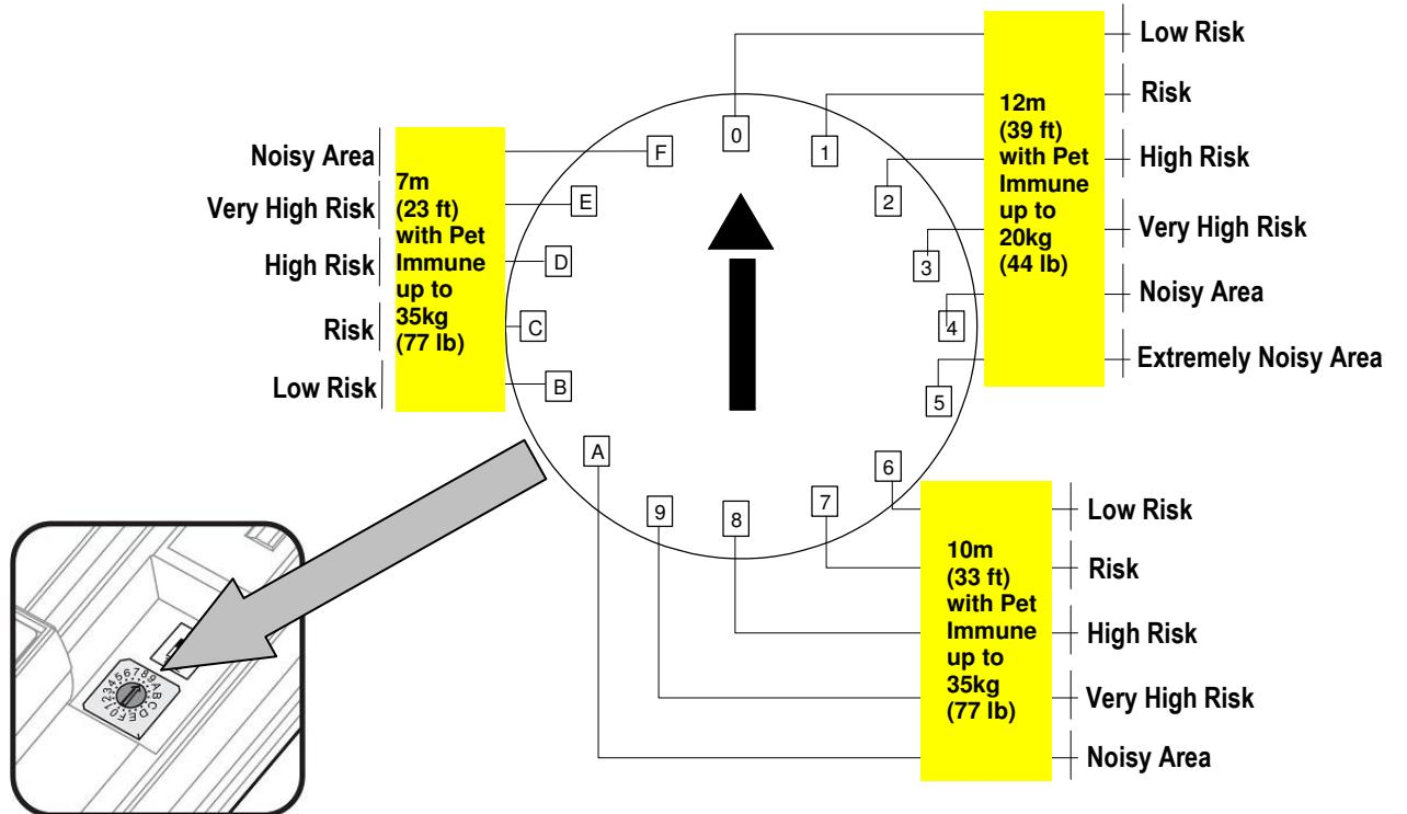
Each group is divided to 5 or 6 sub-positions that help to define the environmental condition inside the detection range:
