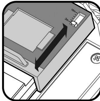
To adjust for ranges between 3m and 12m (10 and 39 ft.) slide the detection element up or down to correspond with the desired distance. Each step between 3m and 12m (10 and 39ft.) represents 3m (10ft) of range.
