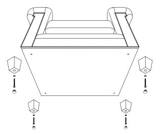
Take down the bag from bottom of chair. The legs are packed inside. Assemble as shown in diagram.
