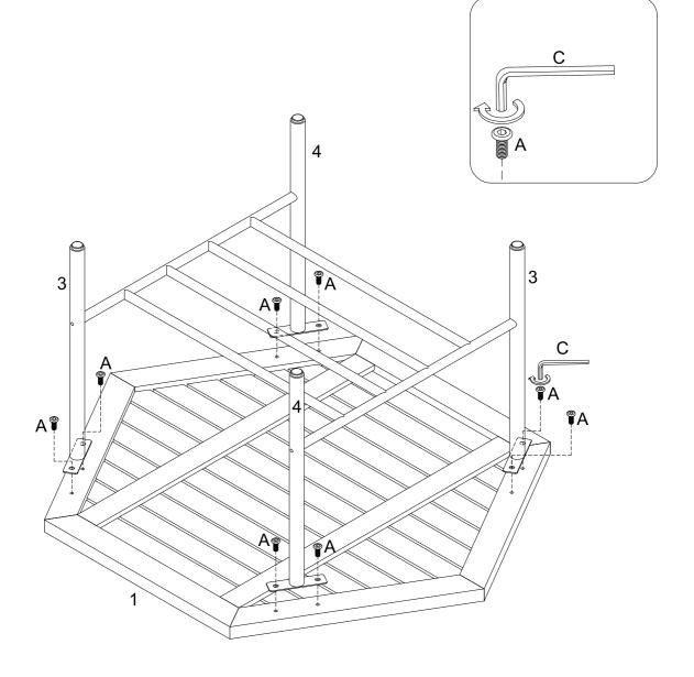
Using bolt (A) attach parts (3,4) to part (1) with Hex key (C) as per diagram. Note:Fully tighten all bolts.
