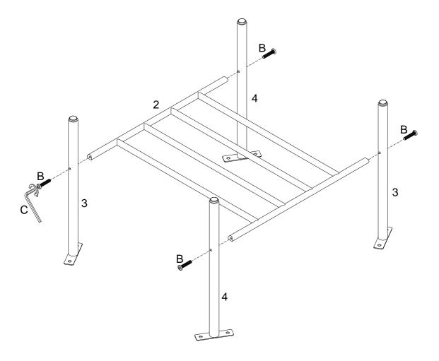
Using bolt (B) attach parts (3,4) to part (2) with Hex key (C) as per diagram. Note:Do not fully tighten all bolts.
